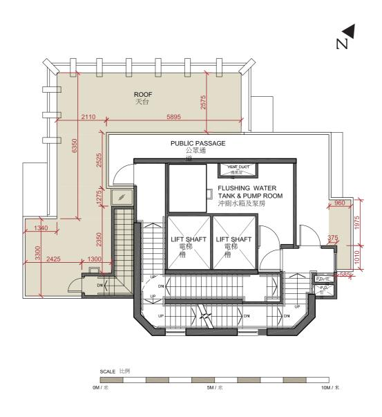
The dimensions in floor plans are all structural dimensions in millimeter.
