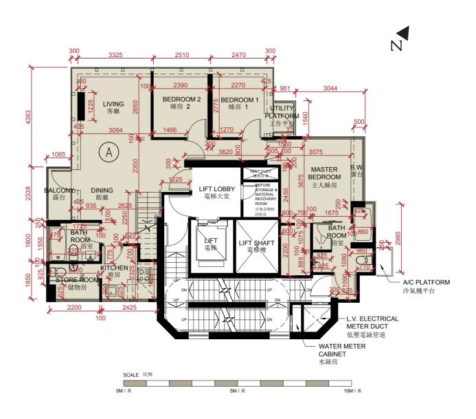
The dimensions in floor plans are all structural dimensions in millimeter.
