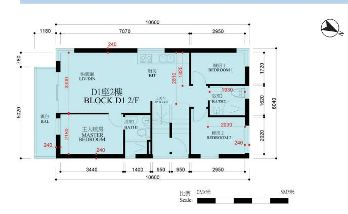
備註:平面圖之尺規所列數字以毫米標示之建築結構尺寸。 Note: The dimensions of floor plans are all structural dimensions in millimeter.
