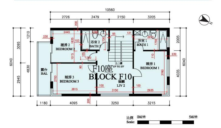
備註:平面圖之尺規所列數字以毫米標示之建築結構尺寸。 Note: The dimensions of floor plans are all structural dimensions in millimeter.
