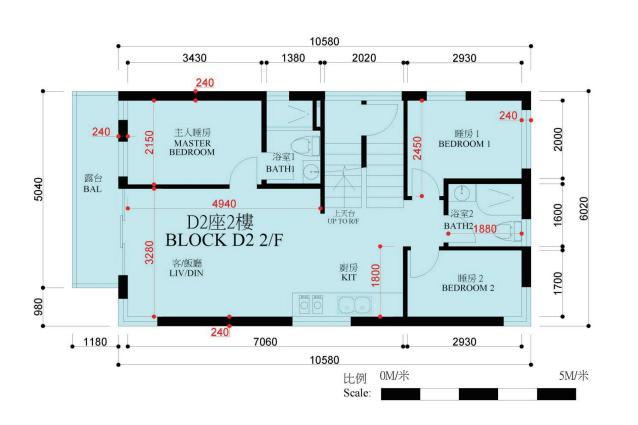
備註:平面圖之尺規所列數字以毫米標示之建築結構尺寸。 Note: The dimensions of floor plans are all structural dimensions in millimeter.
