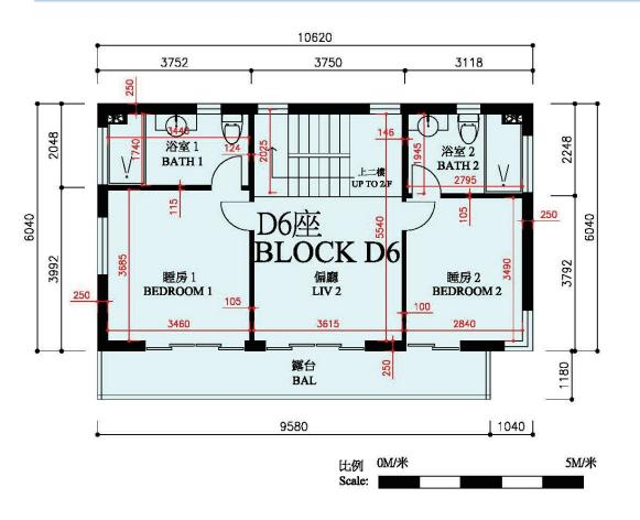
備註:平面圖之尺規所列數字以毫米標示之建築結構尺寸。 Note: The dimensions of floor plans are all structural dimensions in millimeter.
