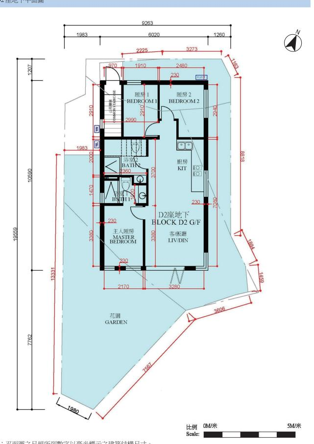
備註:平面圖之尺規所列數字以毫米標示之建築結構尺寸。 Note: The dimensions of floor plans are all structural dimensions in millimeter.
