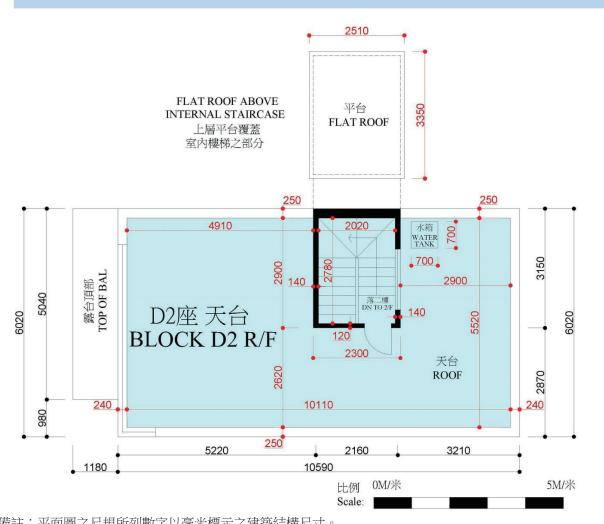
備註:平面圖之尺規所列數字以毫米標示之建築結構尺寸。 Note: The dimensions of floor plans are all structural dimensions in millimeter.
