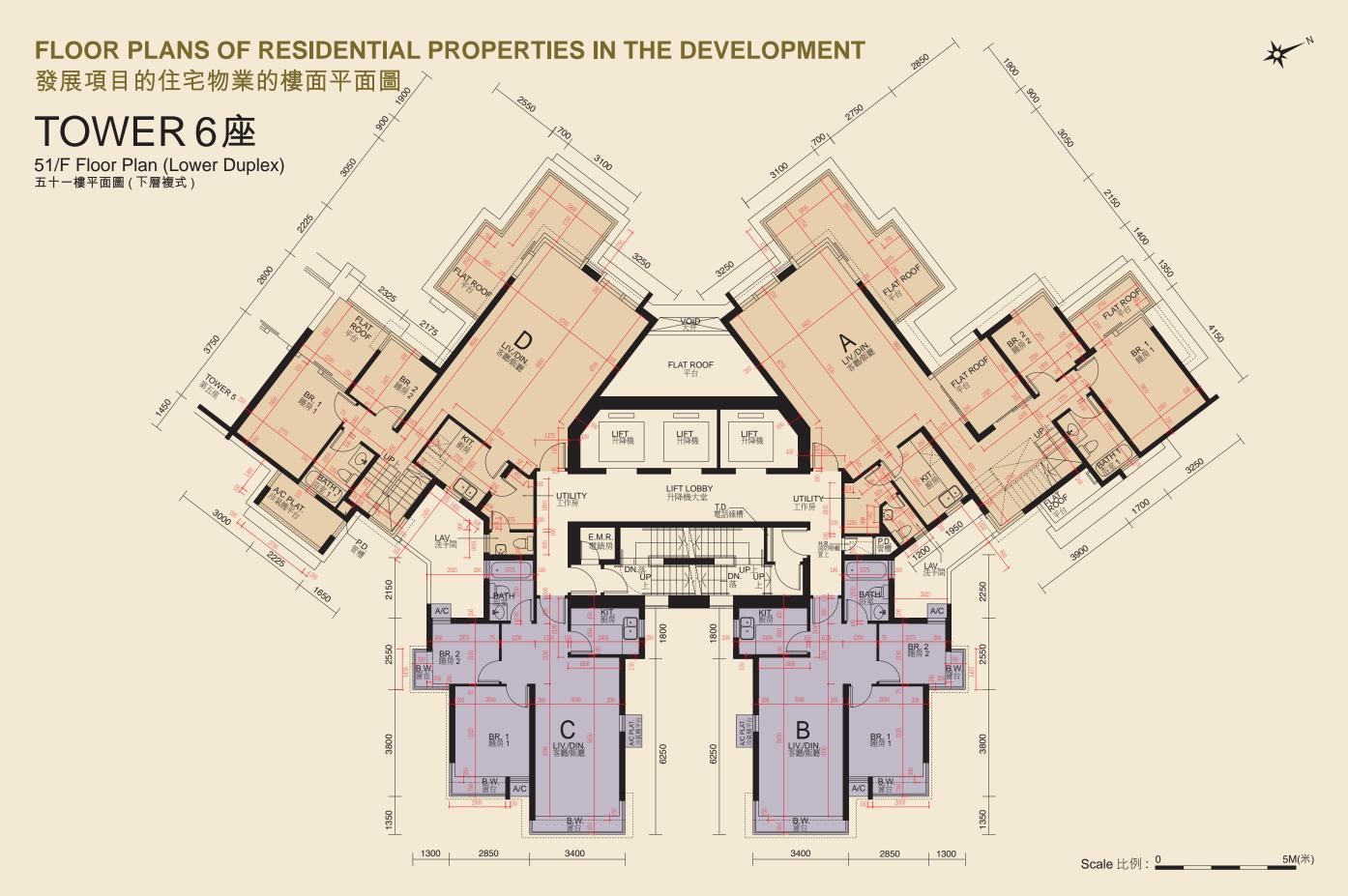
Floor-to-floor height of each residential property as provided in the approved building plans for the development is: typical unit is 3100mm; Duplex unit is 3400mm and 4200mm.
