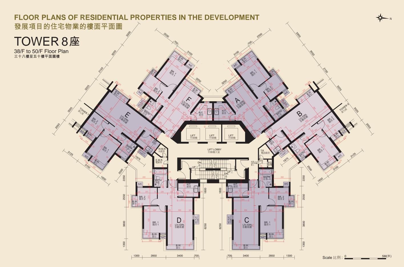
The thickness of the floor slabs (excluding plaster) in the residential properties varies, according to the information set out in the approved structural plans is: 140mm, 200mm and 290mm.
