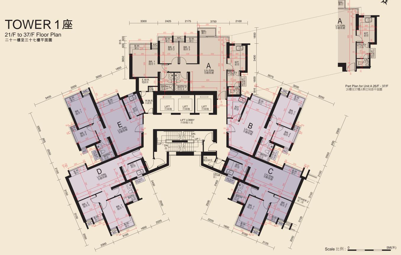
Floor-to-floor height of each residential property as provided in the approved building plans for the development is: 2800mm. The internal areas of the residential properties on the upper floors will generally be slightly larger than those on the lower floors because of reducing thickness of the structural walls on the upper floors.
