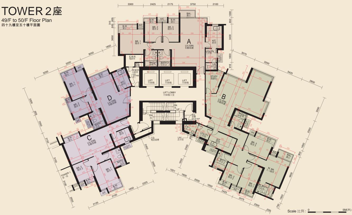
Floor-to-floor height of each residential property as provided in the approved building plans for the development is: 49/F is 2800mm; 50/F is 3150mm.
