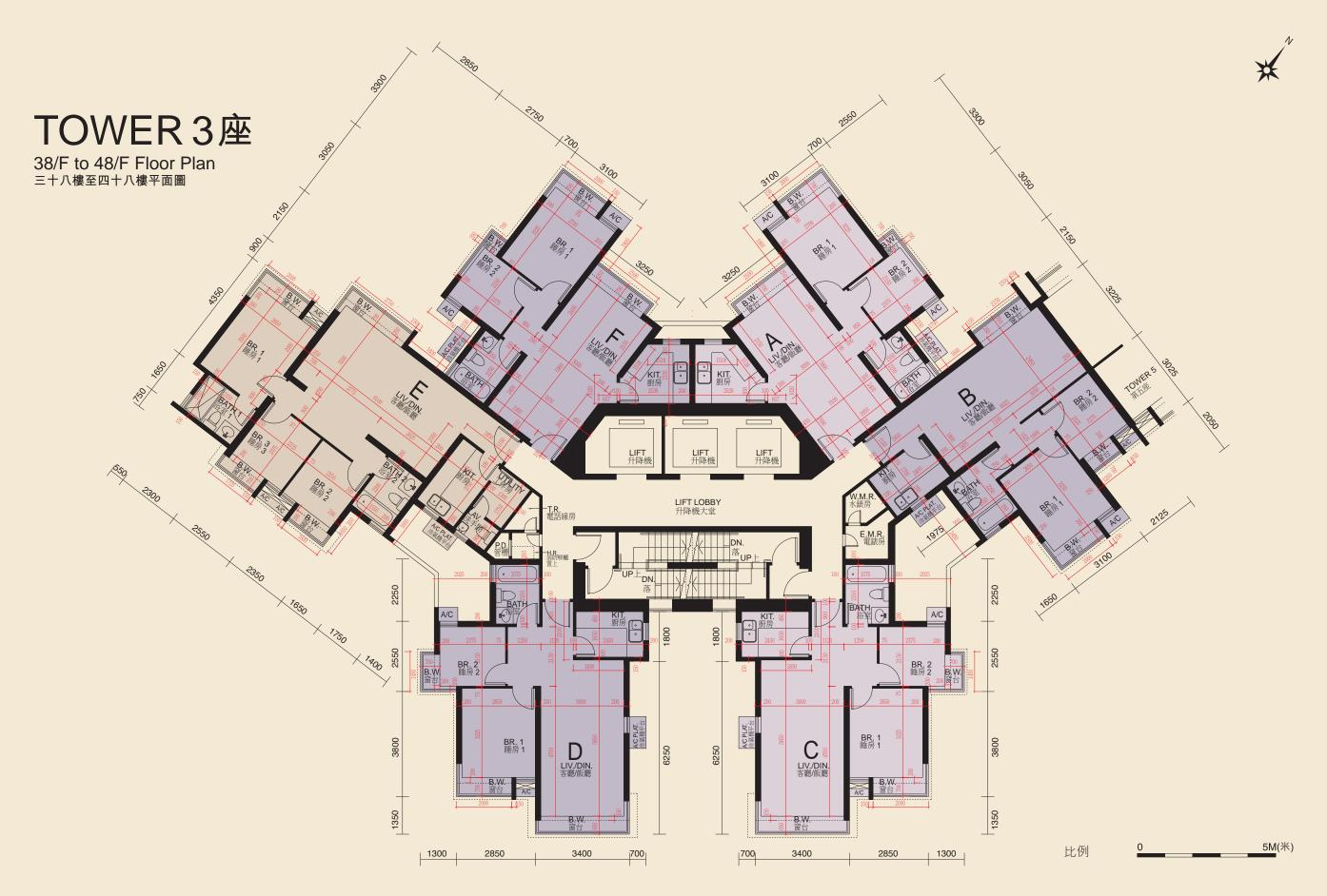
Floor-to-floor height of each residential property as provided in the approved building plans for the development is: 2800mm. The internal areas of the residential properties on the upper floors will generally be slightly larger than those on the lower floors because of reducing thickness of the structural walls on the upper floors.
