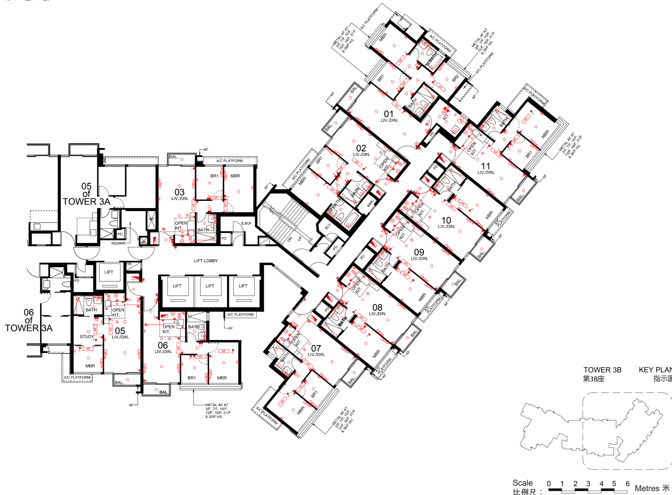
Mechanical and Electrical Provisions 機電裝置說明表
