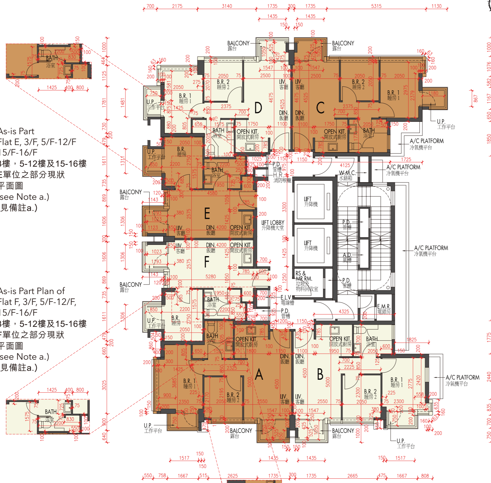
As-is Part Plan of Flat A, 16/F 16樓A單位之部分現狀平面圖 原有浴室門拆除, 安裝新趟門 has been removed and new sliding door Installed.
